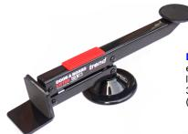
DOOR & BOARD LIFTER Allows up, down, and side to side movement for easy positioning and fixing of doors, panels, and plasterboard. Foot operated lifter to support door while fitting into door frame, freeing up the user's hands. 360 degree rotation. Lifts door 60mm (2-3/8") high and maximum weight 75kg (165lbs). Non-marring foot pad protects floors.
